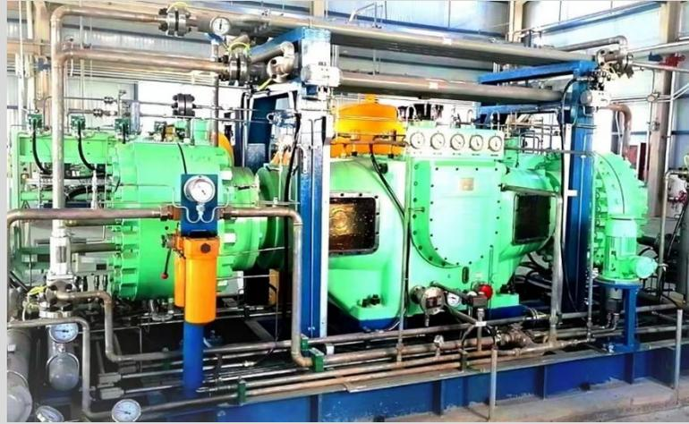
**32MPa filling with diaphragm hydrogen compressor**
